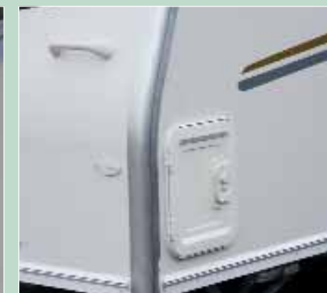
This prototype uses a framework with an awning attachment groove
