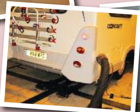
When the Truma Combi boiler is brought into action, fumes from the gas exhaust are removed through a flexible duct. Ice from condensation forms on the body
