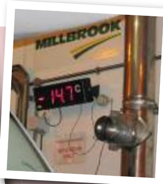
It takes around 10 hours to bring this large enclosure down to -15°C. The progress is monitored for observers to watch on a display screen
