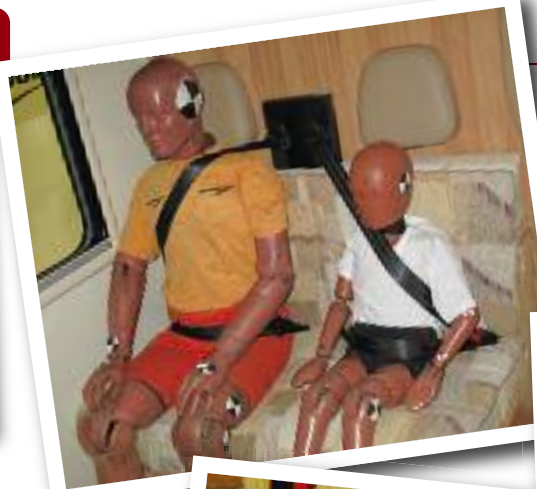
This mock-up uses an SE 760 (six-berth) seating arrangement in which four belted seats are provided behind the driver. The table is removed for the impact test*
