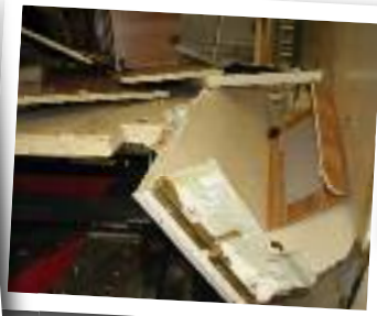
In the first test, a lack of outriggers outside the main chassis rails causes the floor to break lengthways. The fridge and cooker fall out
