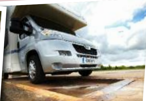
After last winter's frosts, roads were peppered with potholes. At Millbrook Proving Ground, these carefully-crafted obstructions form part of the six-year durability test
