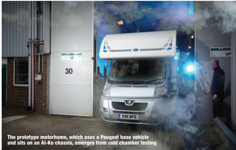
The prototype motorhome, which uses a Peugeot base vehicle and sits on an Al-Ko chassis, emerges from cold chamber testing
