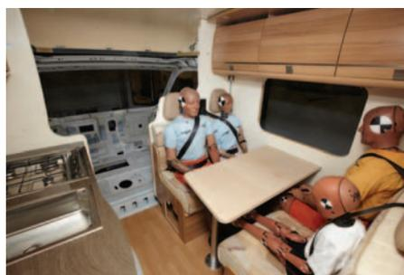
These internal pictures of crash testing reveal four belted rear seats
